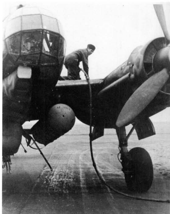
LEFT: Armourers loading LMB 1000 kg parachute mines on the fuselage racks of a He 111. In addition to their intended role of rendering waterways hazardous for shipping, these thin cased weapons were often fitted with impact fuses and employed against land targets.
