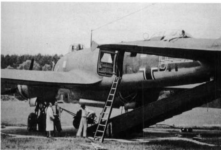
ABOVE: An Fw 200 on the compass swinging base. The transmitting aerials for the little used Neptun S surface search radar can be seen just in front of the tailplane.
