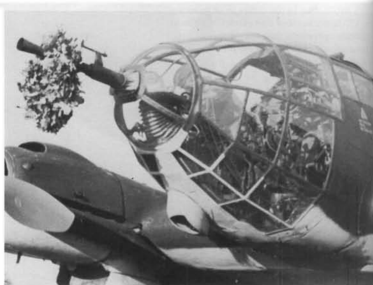
ABOVE: Hans-Georg Bätcher's aircraft suitably decorated on the occasion of his return from his 600th mission. The garland hangs from the barrel of the nose-mounted MG FF 20 mm cannon, with its tapered flash eliminator at the muzzle and external ring-and-bead gunsight.
