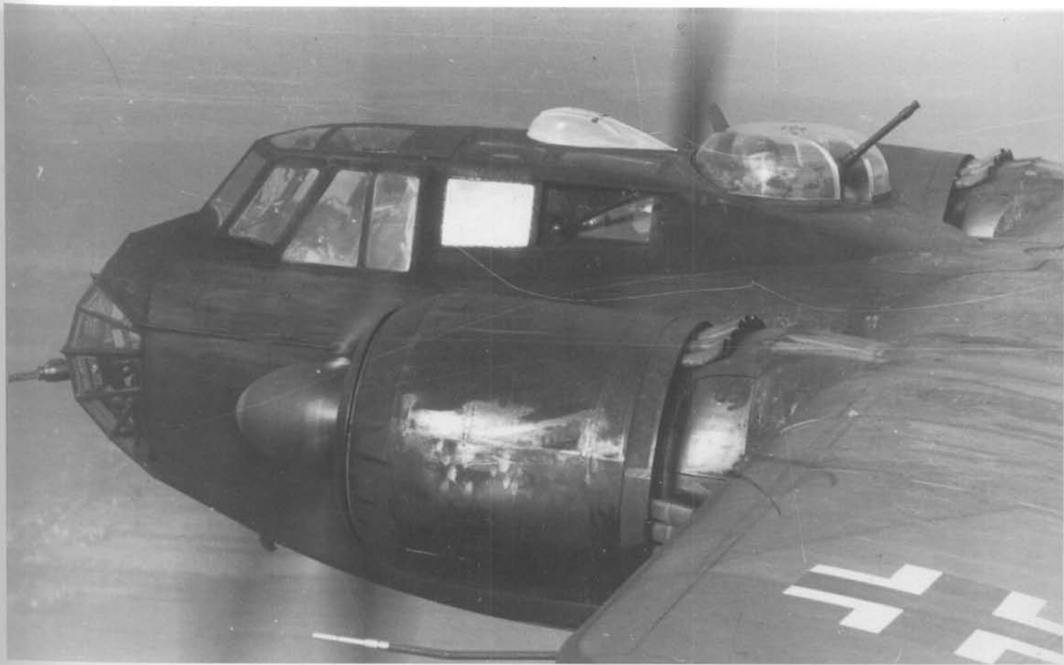
ABOVE: A close-up of the cockpit area of a Do 217 of KG 40, showing the gun turret position fitted with one MG 131 machine gun.
