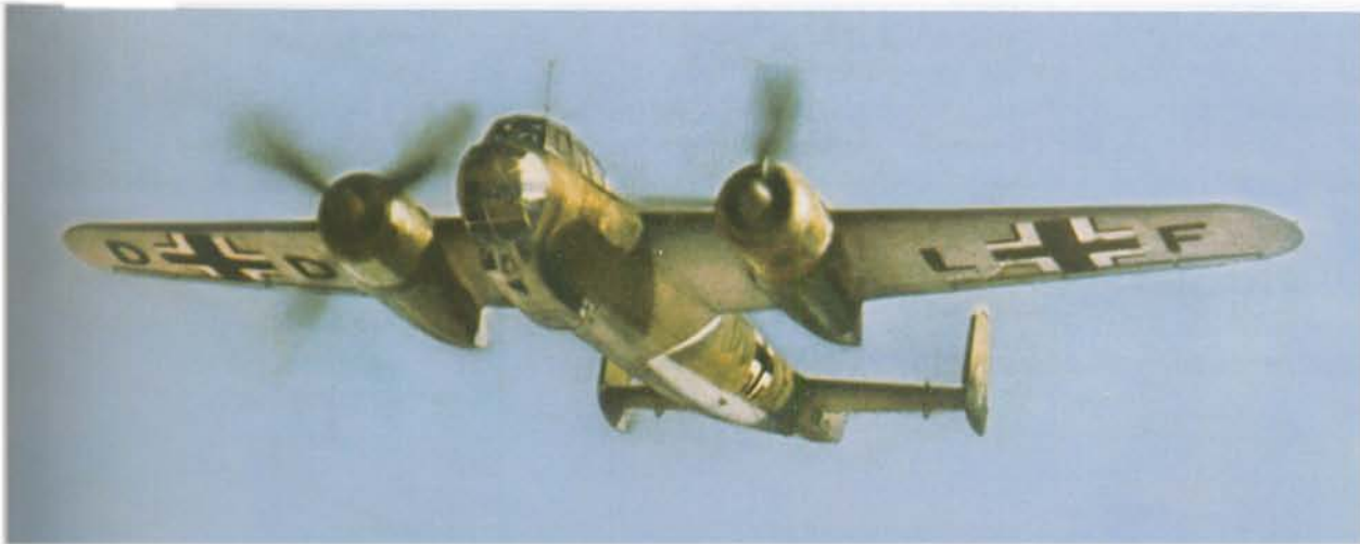
LEFT: This Do 217 E still carrying the factory call-sign DD+LF displays an excellent example of a standard factory finish of RLM 70/71 upper surfaces and 65 pale blue, underneath. The national markings and lettering applied are also to the specified size and location.
