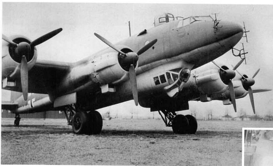
ABOVE: An Fw 200 C fitted with nose-mounted aerials for the Hohentwiel surface search radar.
