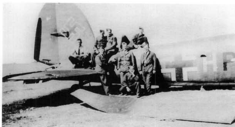
BELOW: This He 111 from 6./KG 26, coded 1H+BP, made an emergency landing on the Spanish coast. Note that the usual white outline to the fuselage cross, swastika and the fuselage band have been overpainted in black for night operations.
