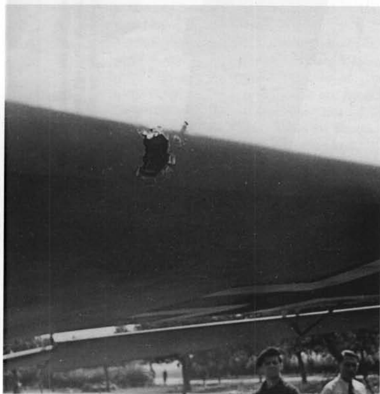
ABOVE AND TOP: The entry and exit holes in the wing of the Ju 86 R caused by the 20 mm round fired by a Spitfire over England on 12 September 1942.
