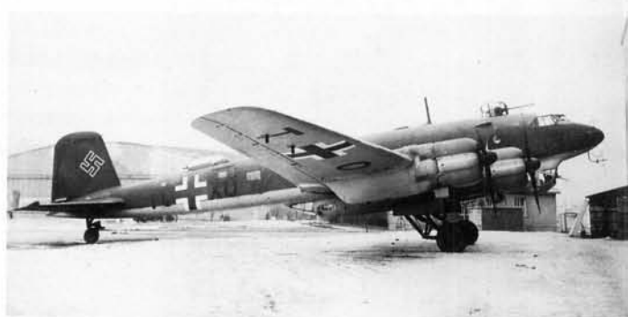
ABOVE: A late production Fw 200 C-8, with deepened nacelles on the outer engines to allow it to carry an Hs 293 missile.
