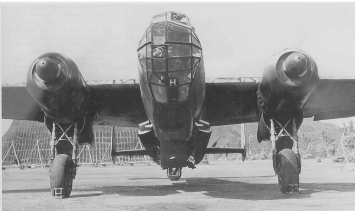
LEFT: A Do 217 E-2 with its bomb doors open, showing the unusual 'double fold' system used on this aircraft.
