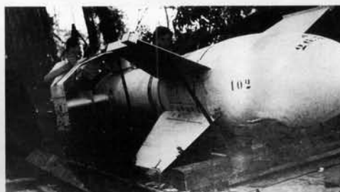
LEFT: A Fritz-X as discovered by the Allies. The photograph gives a good indication of the size of the 1,400 kg (3,100 lb) weapon.
