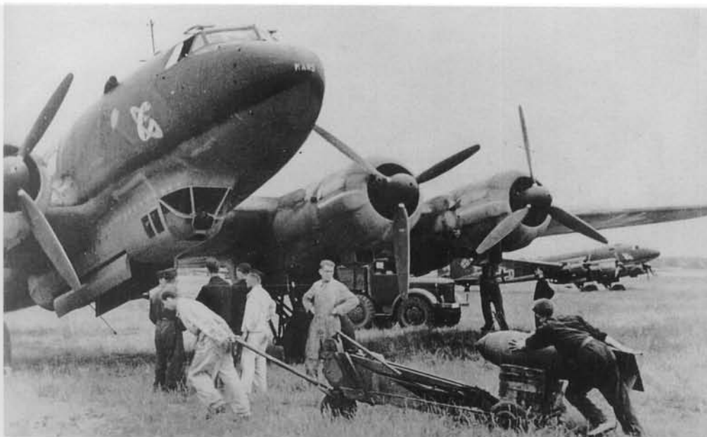
ABOVE AND BELOW: Armourers load SC 250 bombs on Fw 200s of KG 40 at Bordeaux-Merignac. Note the unit's emblem, the 'World in a Ring' painted on the side of the fuselage aft of the cockpit.
