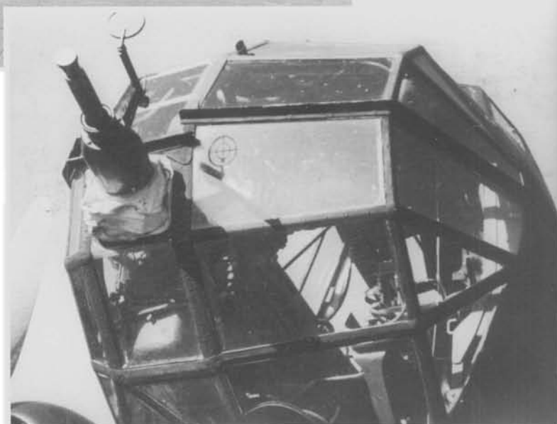
RIGHT: A close-up view of the nose armament of a 20 mm MG FF cannon as fitted to the Do 217 E-5. The weapon was installed to achieve greater operational effectiveness.
