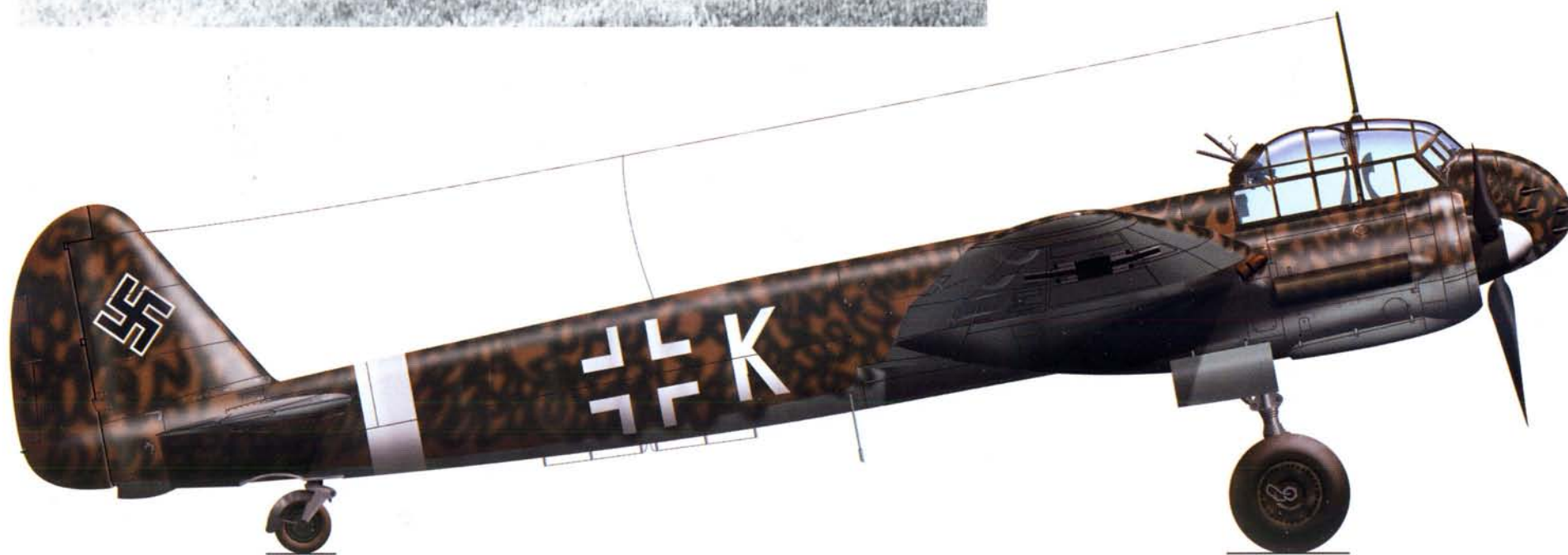
Junkers Ju 88 C-6 of 1./KG 76 based at Catania in Sicily during the early spring of 1943 It has dark green (probably RLM 71) sprayed over its pale blue (RLM 65) finish in a 'scribble' pattern. The white rear fuselage band was carried by most German aircraft operating in the Mediterranean theatre.
