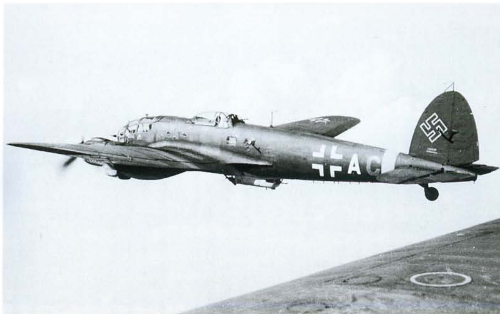
LEFT: A He 111 H-16 of II./KG 53. Just visible protruding from the nose of the aircraft is the 20 mm MG FF cannon carried by these aircraft on the Eastern Front and used mainly for low-altitude ground-strafting missions.
