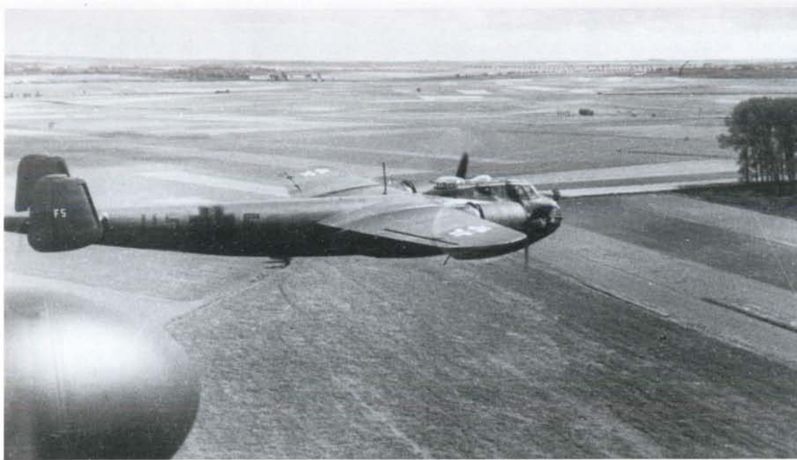
LEFT: A photograph taken in mid-1942 during a mission flying at low level over the French countryside of a Do 217 E-2, U5+FS, of 8./KG 2, seen from another aircraft in the formation. As was common at that time, the undersides and parts of the national markings have been overpainted in black to prevent visibility during nocturnal operations.
