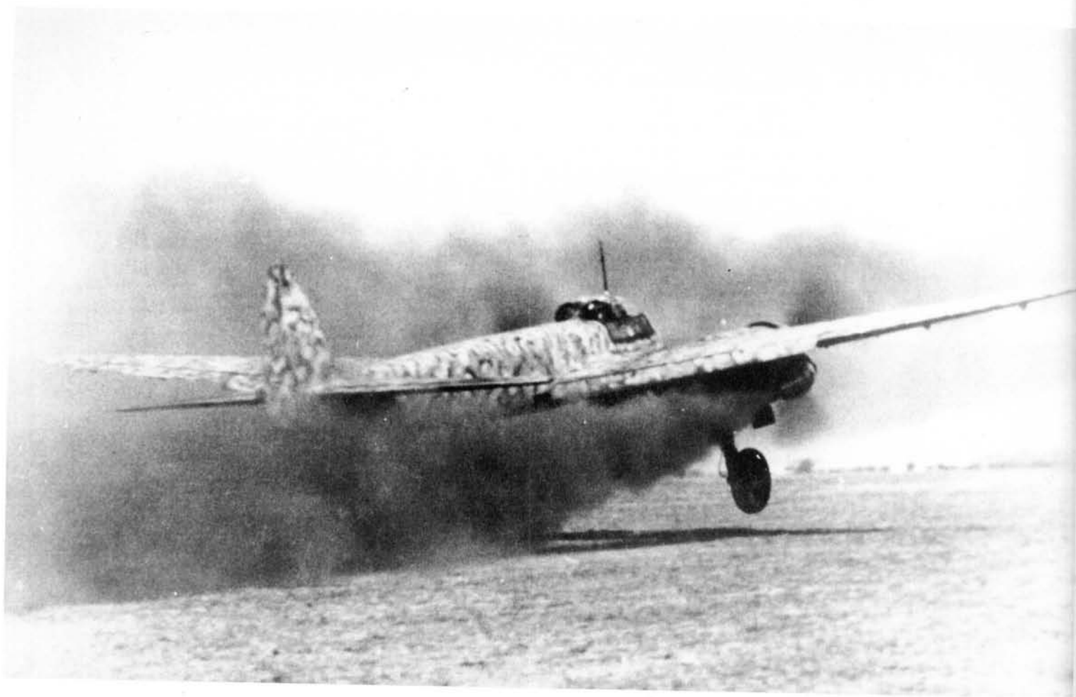
ABOVE AND RIGHT: Using rocket assisted take-off engines this torpedo-carrying Ju 88 from I./KG 77 takes off on a mission over the Mediterranean.
