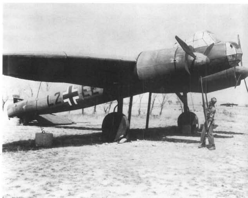
ABOVE: A plywood replica of a Ju 88 set up at the decoy airfield at Salon in the south of France. These decoys were often used to confuse aerial reconnaissance and Allied aircraft.
