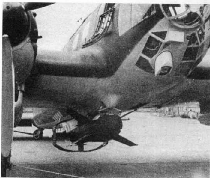
ABOVE: This He 111 H was used by the AVA as a test aircraft for dropping trials of the Fritz-X guided bomb.
